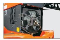
Fan speed can be adjusted depending on fluid temperature to effectively cool down coolant and hydraulic oil. The result is extended component service life and reduction in fuel consumption. The fan is also separate from the engine for easy servicing.
