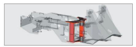
The box-section frame is thickened and strengthened to resist torsion and increase durability. Center pins are widely spaced for higher resistance to torsion.
