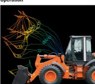
With the parallel/tandem hydraulic circuit, the lift arm and bucket can be operated simultaneously. This is a new function to increase loading and excavating efficiency.
