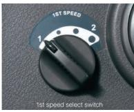
When the first speed range is selected, four travel speeds can be further selected to suit job needs and jobsite conditions. No need for skilful control of the accelerator and brake.
