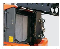
The radiator and oil cooler are made of aluminum instead of conventional steel or copper for corrosion prevention.
