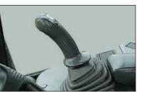
The multi-functional joystick lever is provided atop of the control lever for operating ease.
