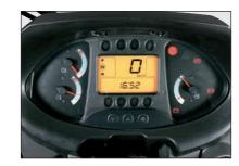
With the easy-to-read monitor, the operator can see instructions for scheduled servicing and maintenance. *Monitor Indication Items:*
