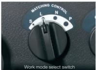
On the ZW140, four work modes are selectable according to job requirements and operator's preference. In each work mode, electronic matching control, originally developed by Hitachi, detects the pressure of the implement, and controls the torque of travel motor to best match traction force and breakout force. This increases production per unit of fuel.
