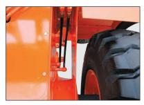
The DL front frame is shaped for easy removal of dirt, stones and snow.
