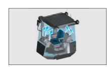
With the front and rear defrosters, airflow comes out from three front air outlets and two rear outlets to protect respective windows from fogging, keeping clear vision even in rain and cold weather.
