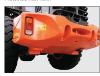
The large counterweight is arranged to protect the fuel tank from collisions with obstacles during operation.
