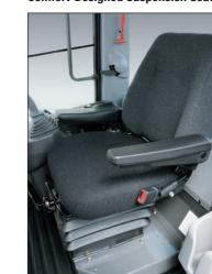
The mechanical suspension seat well absorbs shocks and vibrations from the machine body to reduce operator's physical stresses for enhanced comfort.
