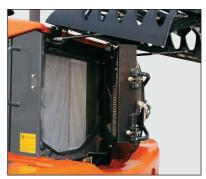
The rotation of the hydraulically operated cooling fan with heat-sensing system is equipped as standard. The fan itself can swing open for easy cleaning.
