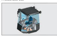
The bi-level air conditioner allows air conditioning at foot space and overhead simultaneously. Airflow volume and direction can automatically be adjusted according to the temperature setting. The pressurized cab shuts out dust and debris even in dusty environment.
