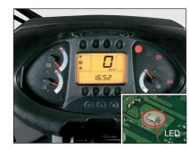
On the indicators, monitors and alarms, many LEDs are utilized for longer service life resulting in less failure, enhancing the reliability.
