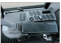
The switches for pre-operation setting are on the right console, and the switches for operation and travel on the front console. They are functionally laid out for ease of operation.
