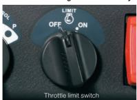
The throttle limit cuts maximum engine speed by 10% for higher fuel efficiency. For the HST system, maximum traction force is not reduced with the reduction in engine speed.
