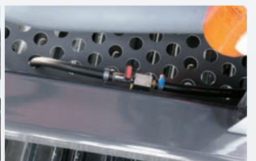
Fuel tank water drainage cock
